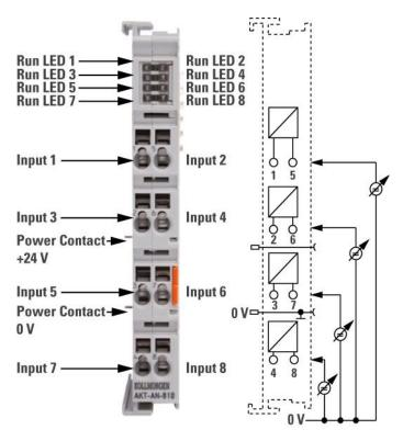
The section describes the connections for the 8-channel analog input terminal.
